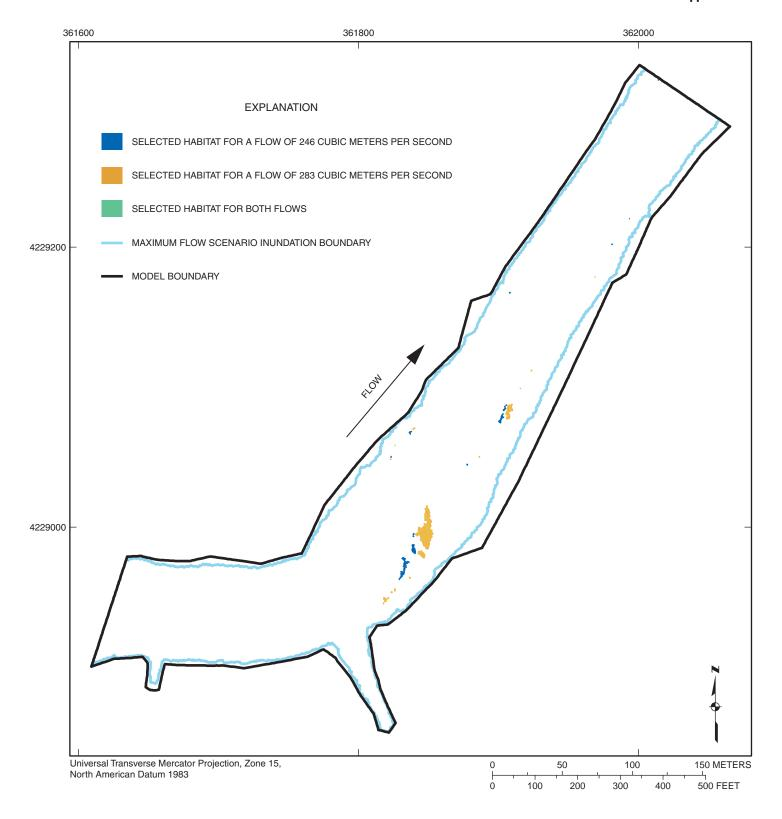
Figure 3-79. Selected habitat area distribution for habitat categories 16, 17 combined (channel catfish) at flows of 246 and 283 cubic meters per second at Marais des Cygnes River site MDC1.
